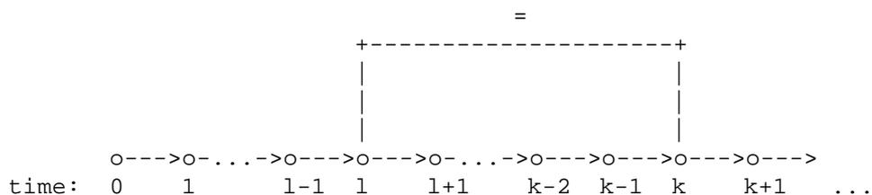
Consider the above figure. It represents an examples of a generic infinite counterexample, with its two parts: the prefix part (times from 0 to  $l - 1$ ), and the loop part (indefinitely from  $l$  to  $k - 1$ ). Because the loop always jumps to a previous time it is called *loopback*. The loopback condition requires that state  $k$  is identical to state  $l$ . As a consequence, state  $k + 1$  is forced to be equal to state  $l + 1$ , state  $k + 2$  to be equal to state  $l + 2$ , and so on.
